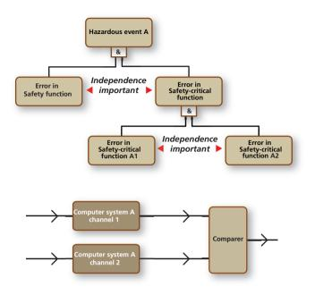
*Figure 4:8 Safety-critical system, multi-channel redundant system (replica)*
