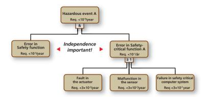
Figure A4:7 Reduced generic field tree, single channel safety critical system
