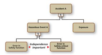
Figure A4:1 General fault tree for break-down of hazardous events
