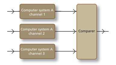
*Figure 4:3 Redundant multi-channel system with three identical computer systems and software with separate input channels*
