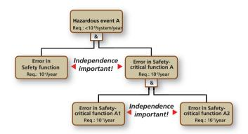
Figure A4:5 Requirement breakdown in safety-critical multichannel diversified system
