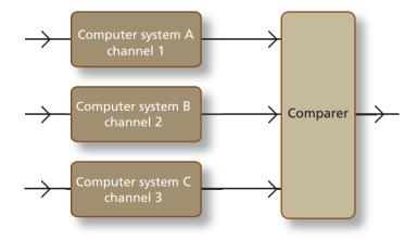
Figure 4:4 Redundant multi-channel system with three different computer systems and three different software and separate input channels
